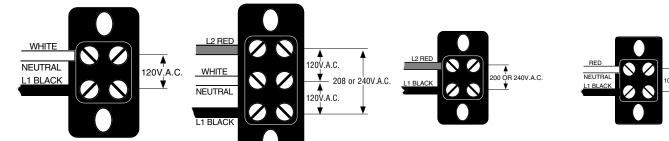
MODELS 0T15 & 20 require 2wire, grounded service rated 120 volts ac, 15 or 20 amp respectively, single phase, 60 Hz. Model 15 has an attached cordset.
