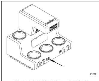
FIG. 21 INDICATOR LAMP - MODEL RT
