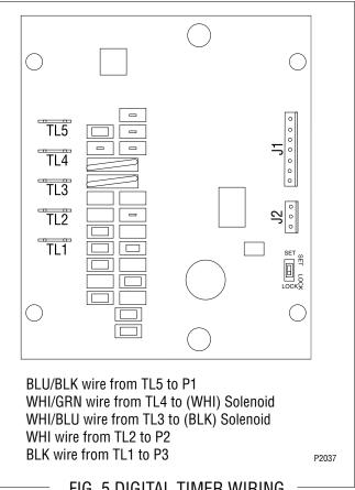
FIG. 5 DIGITAL TIMER WIRING
