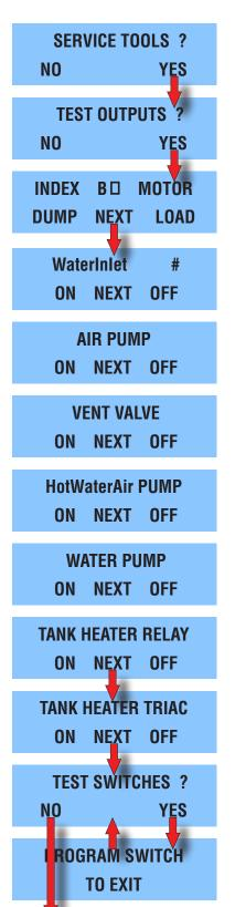
**SERVICE TOOLS** allows testing of load components and switches. **It should only be used by trained technicians.**
