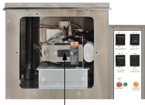
Kettle Circuit Breaker is located behind front cover plate; then remove breaker cover to access the CB.
