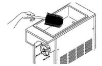
Figure DD Sanitize Hopper
