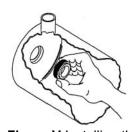
Figure V Installing the stationary half seal
