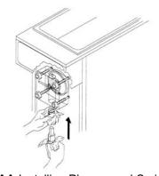
Figure AA Installing Plunger and Spring
