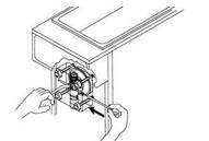
Figure CC Insert Retaining Pin
