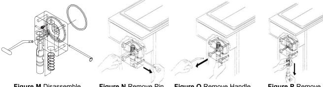
Figure M Disassemble Dispensing Valve
