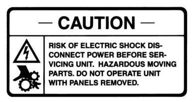
Located on the right, left and rear panels. (part # W0600218)
