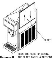
THE FILTER PANEL, & IN FRONT Figure F OF THE EXISTING SIDE PANEL. TO CHANGE, REMOVE, CLEAN AND/OR REPLACE.
