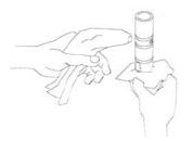
Figure EE Lubricate Carb Tube
