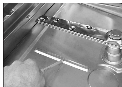
Proper Water Level in the Wash Tank.
