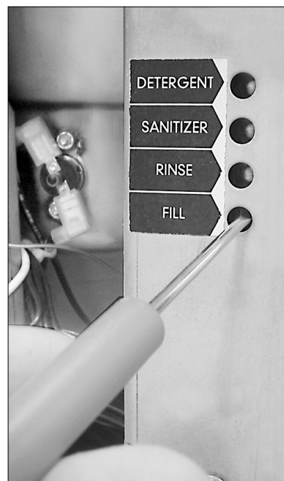
Turning the chemical dispenser adjusting Screws increase or decrease the chemical dispensed.
